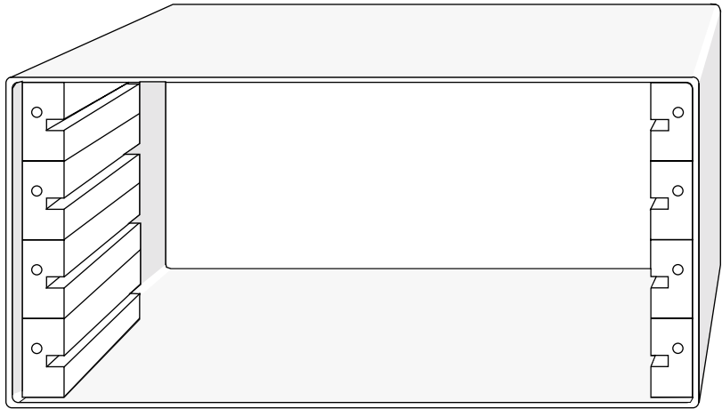
Figure 3-5. ENCL-4 Shell with Four Pairs of Slotted Card Guides (rear panel not shown)
